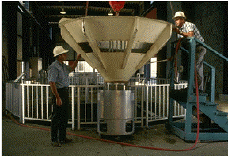
Photograph J-8. View of the Skinner Fish Facility Bucket and Counting Station The bucket is positioned at the counting station. (Source: California Department of Water Resources.)
